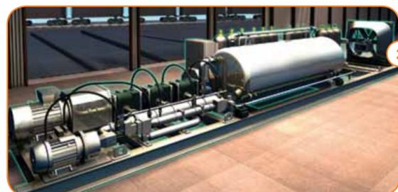
**2 Hydraulic system for coal off-loading**
